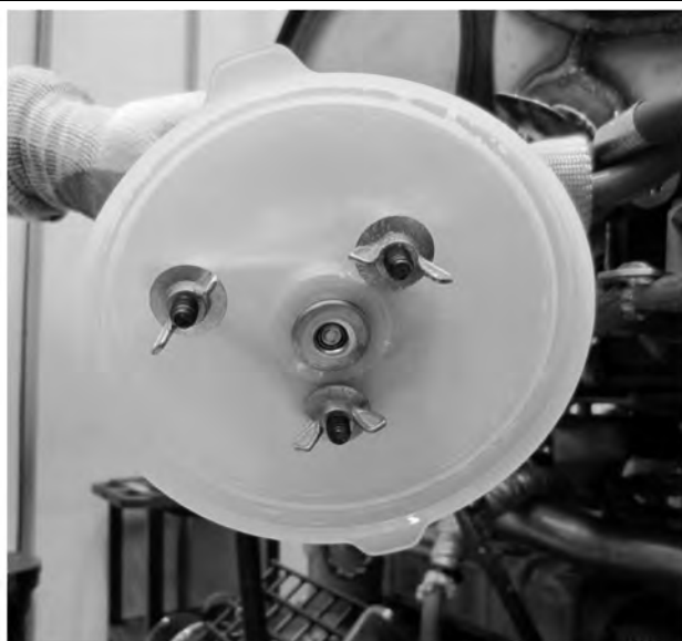
Illustration 100 g03370846 DEF injector bolted to measuring container lid
